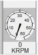
6. Once the spindle has reached 0 RPM; close the spindle cover and lock, <u>remove the interlock key</u> and close the dicing saw cover fully.
