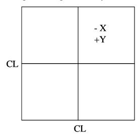
mark placed in quadrant 1 on the mask. The picture assumes normal Cartesian coordinates with the center lines crossing at 0,0 and the mask is chrome-side down and oriented as it would be on the stepper. (This is the same orientation that you will have when viewing your LEdit file)
