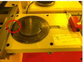
7. Locate the needle valve on the right side of the stage, behind the X-axis stage micrometer. Turn the needle valve knob clockwise until it stops.
