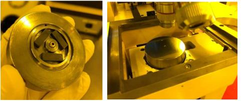
**NOTE:** There are 2 holes on the top of this chuck spacer, one in the center and one offset from center. <u>The orientation of the offset hole DOES NOT MATTER</u>.
