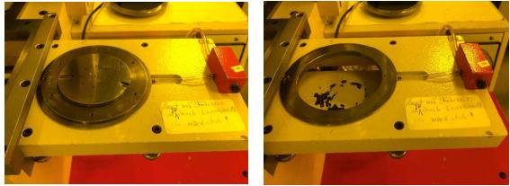
4. Disconnect the chuck adapter ring vacuum line from the transport slide by pulling it off of the barbed connection on the transport slide (red block). Do not remove the vacuum line from the chuck adapter ring!
