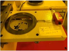
6. Select the desired topside alignment chuck and insert it in the chuck adapter ring, making sure to orient the chuck so that it sits in the pin on the left side of the adapter ring.
