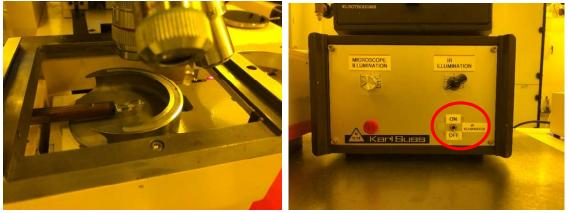
2. With the chuck transport slide out (to the right) remove the backside alignment chuck spacer from the stage by lifting it off.
