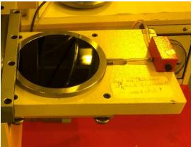
7. Locate the needle valve on the right side of the stage, behind the X-axis stage micrometer. Turn the needle valve knob counterclockwise until it stops.
