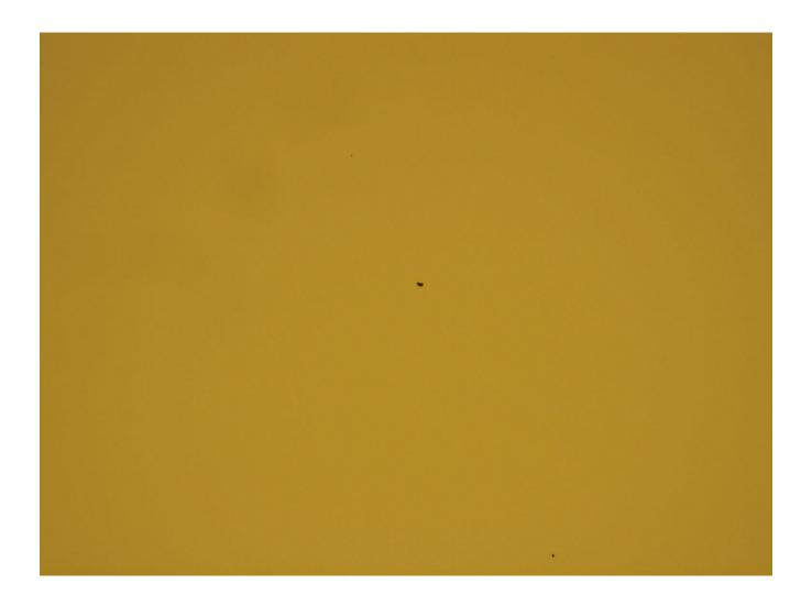
4) a-Si film deposition on the customer's thermal oxide/Si wafer with 5mT, 12.5/400W, SiH4/Ar/He flow-rate=10/20/200 sccm, and time=2593 seconds.
