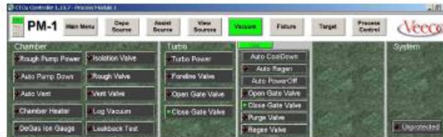
Figure 3-19. Vacuum Control Panel
