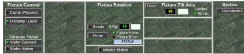
Figure 3-22. Fixture Control Panel
