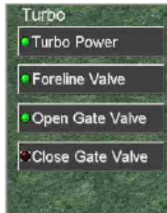
Figure 3-20. Turbo Pump Controls
