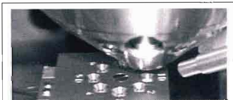
FIGURE 9-1 THE STEM DETECTOR ON A XL30 STAGE
