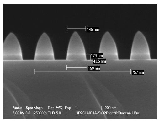
Note: The SiO2 was over-etched into Si as seen in above figure.
