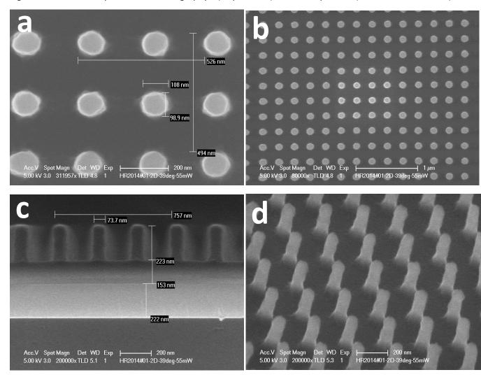
Figure 1. 2D-dot resist pattern after Holography. a) top view; b) another top view; c) cross-section view; d) 45° view.
