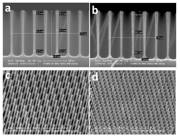
The averaged diameter of the nanowire is 42.3 nm.
