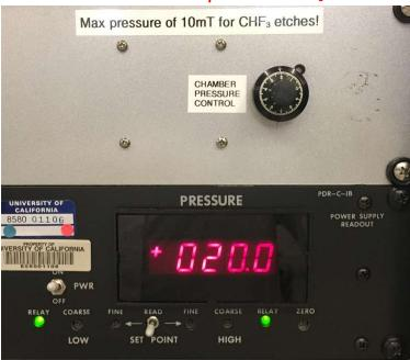
**NOTE:** If you adjust the chamber pressure up too fast, you may exceed the upper chamber pressure set point (110 mT) and cause the HI-VAC valve to close. Decreasing the chamber pressure at this point will do nothing as there is no pumping on the chamber occurring. To rectify this, do the following:
