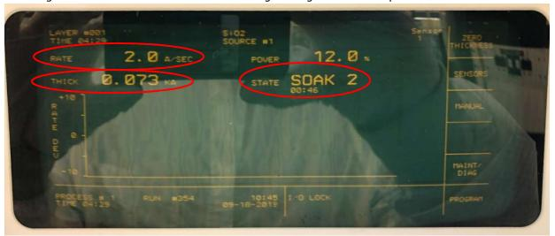
31. Once the Deposit step begins, the shutter will open and the THICK reading will be zeroed out. The controller will begin adjust the power to achieved the rate specified in Step 22. Also, the Rate Dev line chart on the display will begin to graph in real-time.
