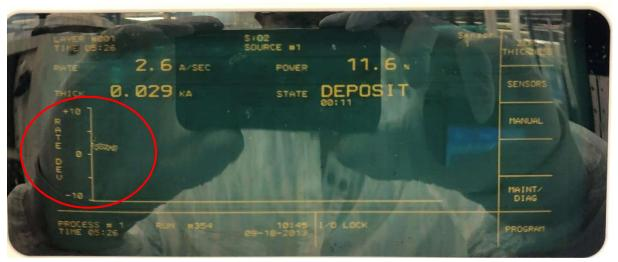
32. Modifying the generic processes is not allowed, however a user can switch a generic process to manual mode if, for example, the system is taking too long to get the rate in control. This is performed as follows:
