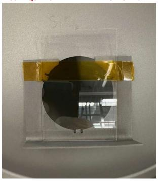
6. Remove the sample holder you require, non-heated or heated, from its holding fixture. If you are using the heated sample holder, you must also remove the non-heated sample holder and leave it out during your run.
