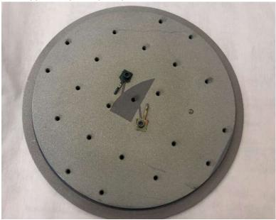
For the heated holder, mount your samples <u>or full wafer</u> on the supplied TOX wafer. Use the 1/16 Allen wrench/driver to loosen the Inconel clip screws and always use the blue handle torque driver to tighten them. The Inconel sample clips must be in <u>all 8</u> positions as pictured below.
