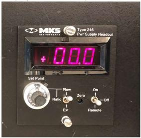
18. Move the other switch up to the On position and begin to introduce gas into the chamber by slowly turning the Set Point dial clockwise. When introducing gas into the chamber do it in increments of 5 SCCM at a time, waiting for the chamber pressure reading on the chamber gauge to drop or stabilize each time before proceeding.
