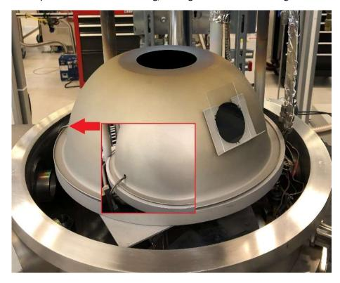
Place a 75 x 50 mm glass slide, standing on its shorter edge, on the front of the dome tooling and secure it with Kapton tape. These are the larger glass slides in the lab.
