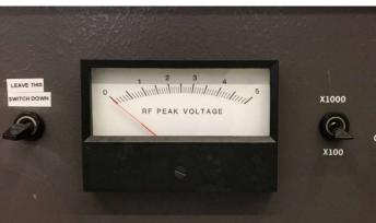
**NOTE:** The multiplier switch next to the meter adjusts the scale of the meter, in most cases X100 is adequate.
