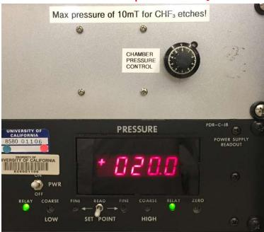
**NOTE:** If you adjust the chamber pressure up too fast, you may exceed the upper chamber pressure set point and cause the HI-VAC valve to close. Decreasing the chamber pressure at this point will do nothing as there is no pumping on the chamber occurring. To rectify this, do the following:
