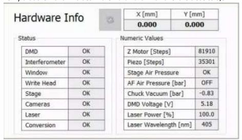
The amount of tolerance for these values will depend on your sample size. For example, if your sample is 10 x 10 mm, then a value of >4 mm (for X or Y) could potentially create a situation where the head could crash. To rectify this, you will need to initialize the stage as follows:
