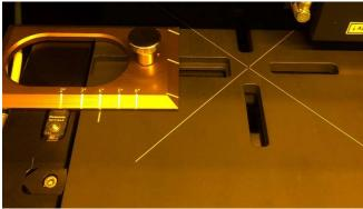
8. Place your wafer on the chuck and press the <u>Wafer Flat to the Left</u>, against the alignment fixture as shown.
