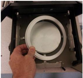
9. Place the inner/smaller hoop of the 7" hoop set around the adapter. The hoops have a rounded edge and a sharper edge. The rounded edge must be facing up for the inner hoop, as shown in the sketch below.
