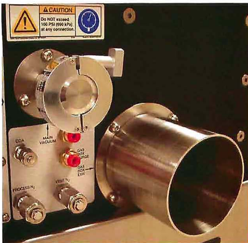
Figure 8. Close-up of Gas, Vacuum, and Exhaust Connections.
