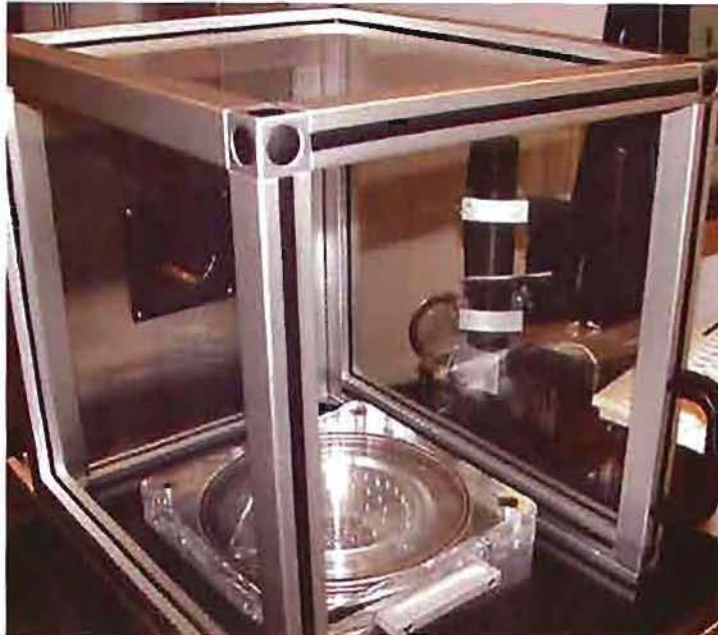
Figure 15. Chamber ventilation shroud pulled forward.
