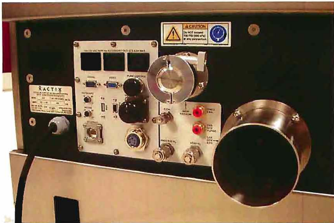
Figure 6. Rear Connections of Xactix. Note, some systems may have different sized exhaust connections. Contact XACTIX for specific information.
