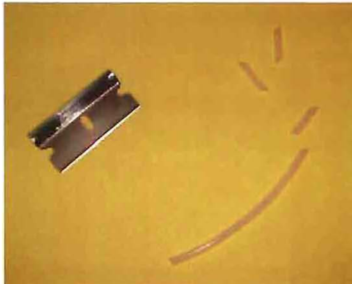
Figure 23. Teflon beading and pieces that have been cut from it using a razor blade.
