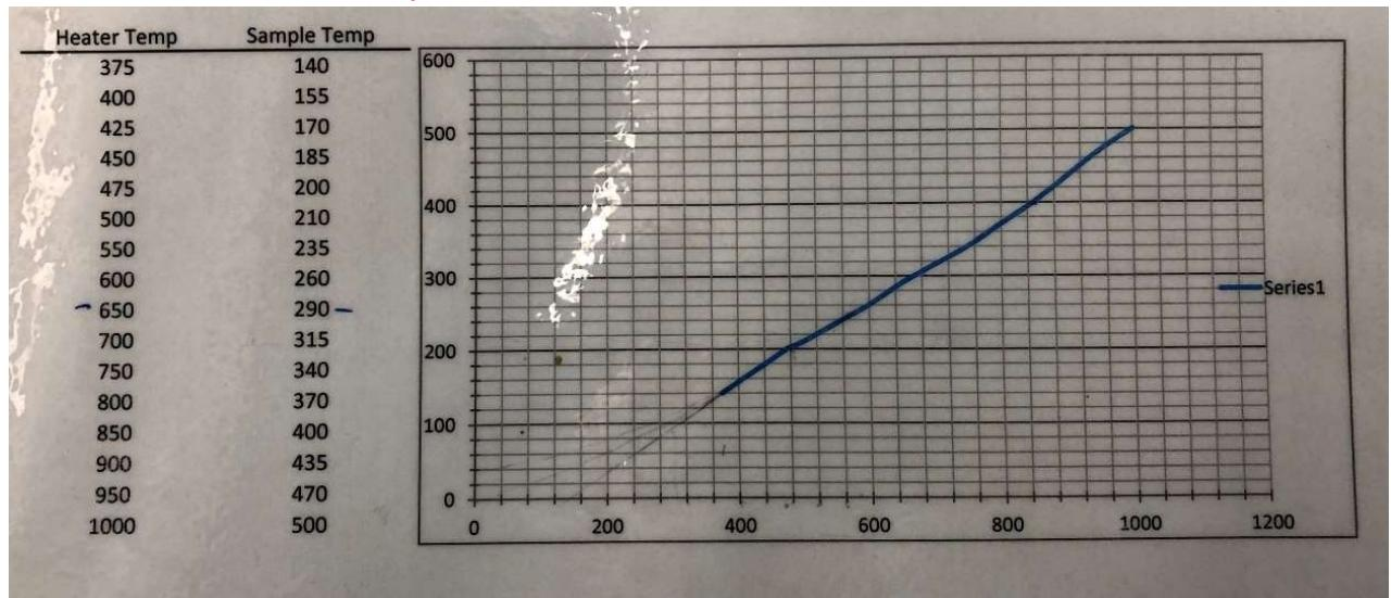
**IMPORTANT:** The maximum the heater can be set to is 700°C! Any temperatures above that require Staff approval.
