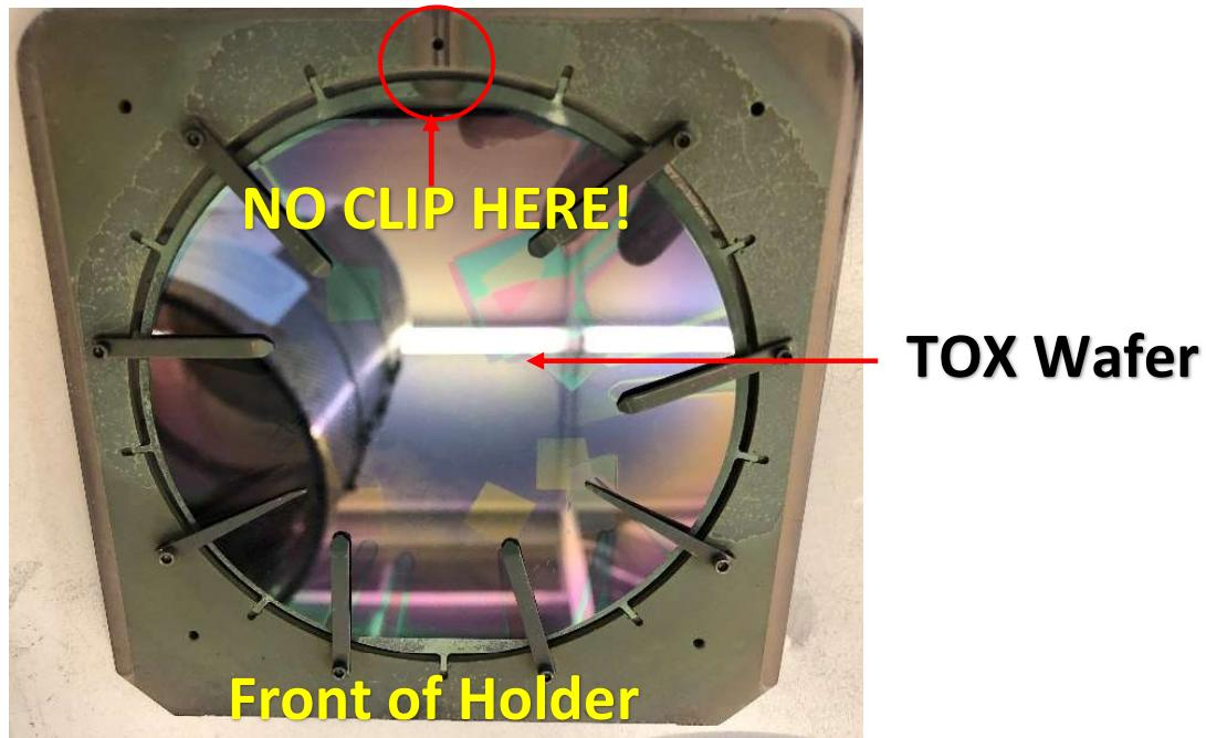
**IMPORTANT:** There is a 9<sup>th</sup> clip position circled in red above. DO NOT place a clip in this position as it will interfere with the thermocouple contact and damage it!
