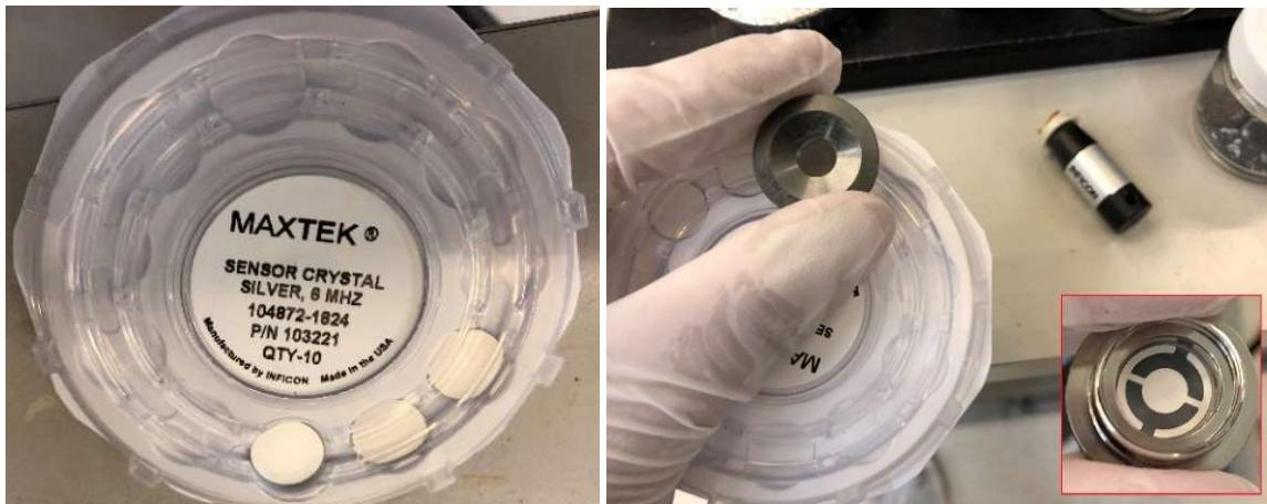
v. Using the Crystal Snatcher, re-install the ceramic retainer into the sensor head. Once it is properly seated, use a slight side-to-side motion to release the Crystal Snatcher. Now, using the bottom of the Crystal Snatcher, press on the ceramic retainer to ensure it is seated properly.
