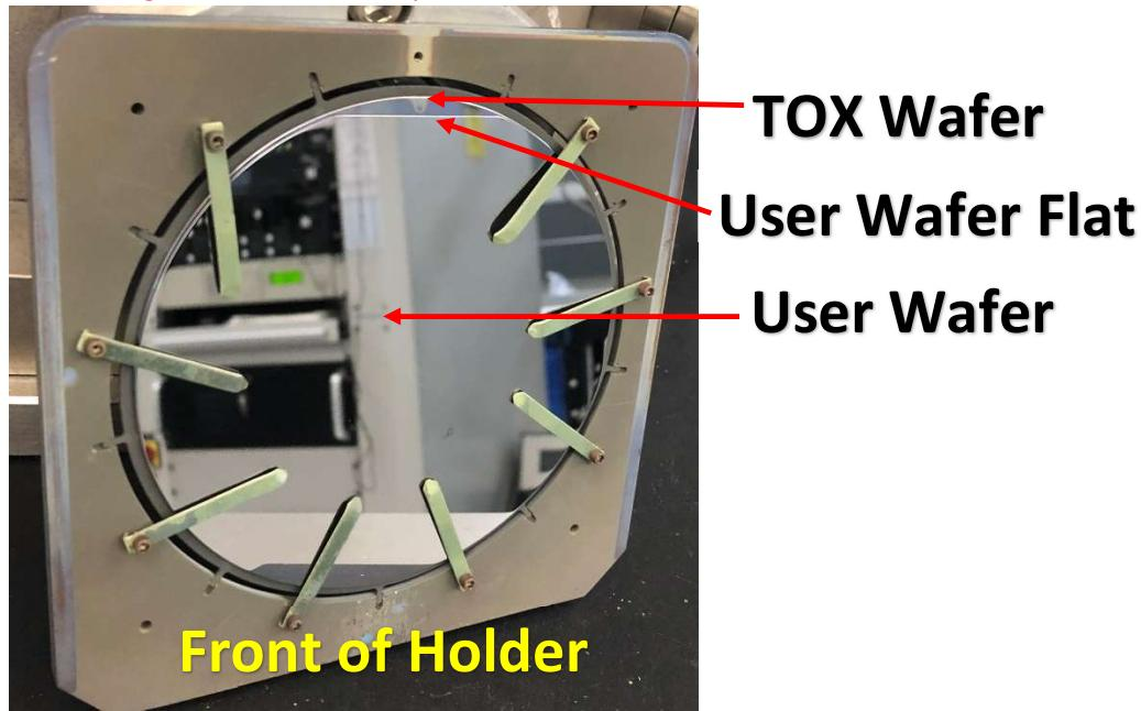
8. Return the sample holder to its holding fixture. The heated sample holder must be slid in uniformly. If it gets stuck, slide it back out and try again.
