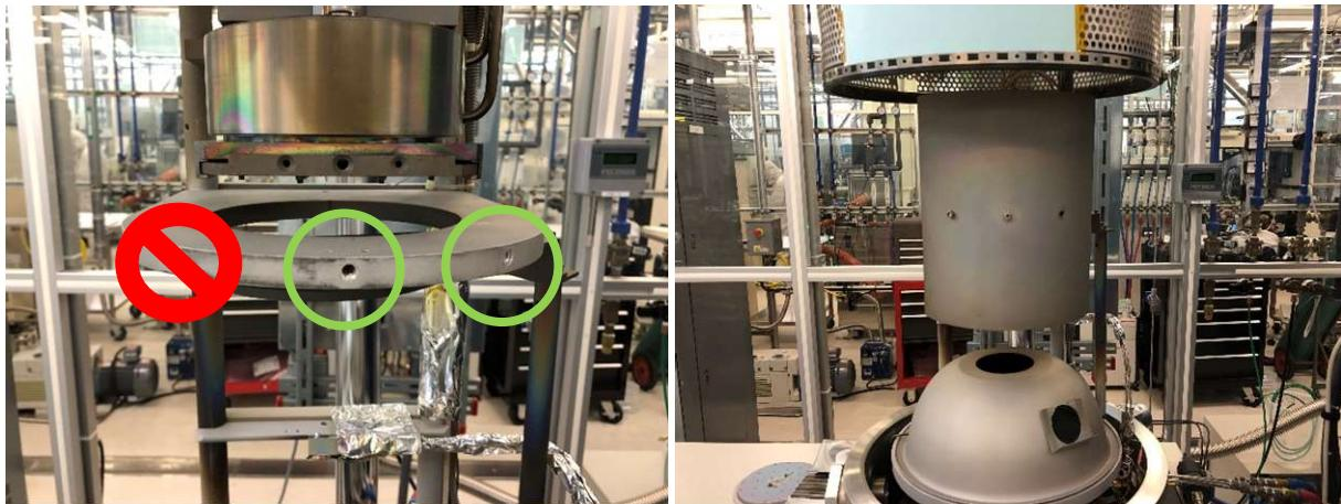
10. Inspect the sealing surface of the bell jar for any flaking or foreign material. Clean this surface with IPA and a wipe as needed.
