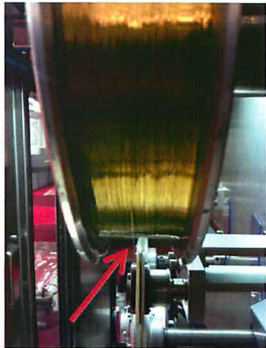
Wire is not straight to pulley (X)
