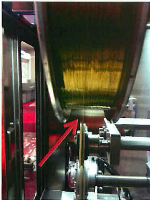
Wire is straight to pulley (O)
