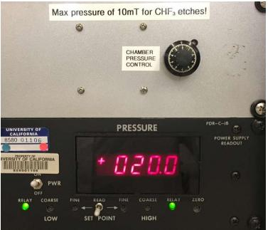
NOTE: The maximum chamber pressure for CHF<sub>3</sub> etches is 10 mT!
