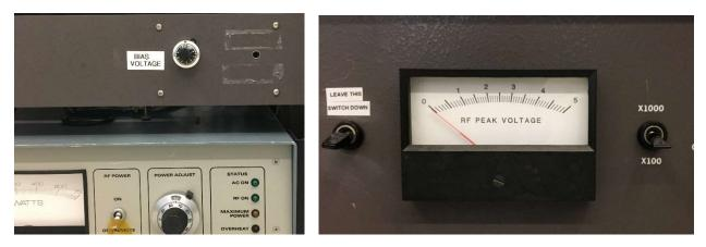
**NOTE:** The multiplier switch next to the meter adjusts the scale of the meter, in most cases X100 is adequate.
