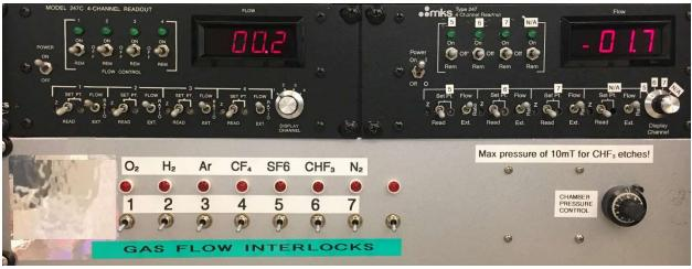
NOTE: The maximum flow rate for SF<sub>6</sub> is 15 sccm!
