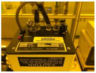
5. Open the small panel on the front of the IR camera monitor and move the POWER switch to the ON position.
