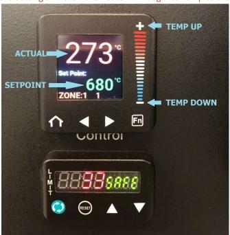
**IMPORTANT:** The setting you set the heater to is not what the sample temperature will be, you will need to reference the **Temperature Offset Table.**
