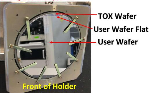
9. Return the sample holder to its holding fixture. The heated sample holder must be slid in uniformly. If it gets stuck, slide it back out and try again.
