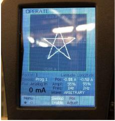
h. You are allowed to adjust the sweep parameters (size, shape, frequency and position), but you are not allowed to save your changes when you are finished. As soon as you make any change to a sweep program, both the handheld and EBC screens will read Editing. After your run is completed or if you decide to change the program, <a href="ALWAYS select Exit Edit">ALWAYS</a> select Exit Edit to ensure the changes you made were not saved to the program.
