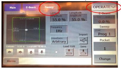
22. From the main OPERATE screen on the IC5, select PROGRAM (F6) and then select PROCESS DIRECTORY (F2). Using the arrow keys, scroll to the desired Process # that has the material(s) you want to run and select PROCESS (F5).
