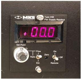
19. Move the other switch up to the On position and begin to introduce gas into the chamber by slowly turning the Set Point dial clockwise. When introducing gas into the chamber do it in increments of 5 SCCM at a time, waiting for the chamber pressure reading on the ion gauge chamber gauge to drop or stabilize each time before proceeding.
