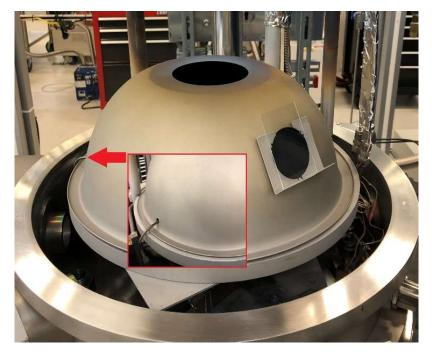
Place a 75 x 50 mm glass slide, standing on its shorter edge, on the front of the dome tooling (these are the larger glass slides in the lab). THIS IS VERY IMPORTANT AS FAILURE TO DO SO WILL RESULT IN COATING OF THE BELL JAR, MAKING VEIWING THE BEAM POSITION EXTREMELY DIFFICULT AND IT WILL REQUIRE STAFF MAINTENANCE TO FIX!
