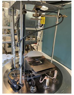
2. Using both hands, plug in the male plug on the cable to the female plug in the chamber. The plug only
