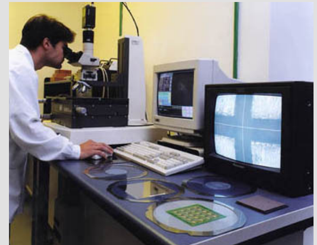
Internal quality analysis on XY Measuring Microscope
