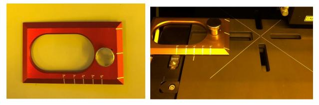
8. Place your wafer on the chuck and press the <u>Wafer Flat to the Left</u>, against the alignment fixture as shown.
