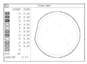
Figure 2. 300-RPM Dynamic dispense (3 seconds). 3000 RPM (12 seconds). 6 inch wafer. Pre Coat Particle Count – 25 (Particles 0.2pm). Total Particle Count – 36. Actual Particles Added - 11.
