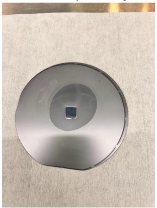
7. Remove the coupon from the silicon wafer by pushing the coupon sideway until it slides out of the silicon.
