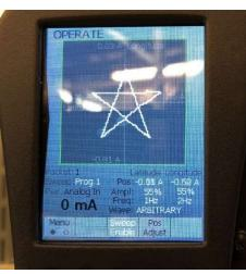
h. You are allowed to adjust the sweep parameters (size, shape, frequency and position), but you are not allowed to save your changes when you are finished. As soon as you make any change to a sweep program, both the handheld and EBC screens will read Editing. After your run is completed or if you decide to change the program, <a href="ALWAYS select Exit Edit">ALWAYS</a> select Exit Edit to ensure the changes you made were not saved to the program.
