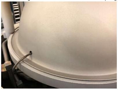
**NOTE:** Before performing the following steps, you may want to use a vacuum cleaner to clean up any flaking. Additionally, there is a wire brush at the system that can be used to remove deposition build-up from the turret pocket(s).
