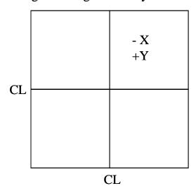
mark placed in quadrant 1 on the mask. The picture assumes normal Cartesian coordinates with the center lines crossing at 0,0 and the mask is chrome-side down and oriented as it would be on the stepper.
