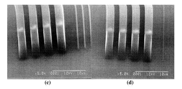
**Note:** The resist thickness is ~7.0  $\mu$ m. In this range of focus offsets and exposure times, the resist will image 1um designed openings as 1.25 um openings in the resist. 1um actual spaces can be realized for the larger focus offsets and exposure times. More room may be available if a positive focus offset is used.
