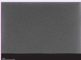
800 nm squares, 1200 nm pitch, imprinted in mr-UVCur06, large-area imprint (Courtesy of Profactor)
