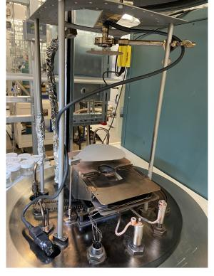
2. Using both hands, plug in the male plug on the cable to the female plug in the chamber. The plug only fits one way.
