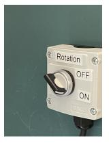
4. When the deposition is complete, Turn the switch off to turn off the rotation.
